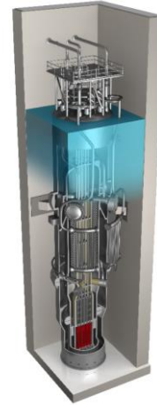
Figure 24. NuScale Power Module (courtesy of NuScale)
